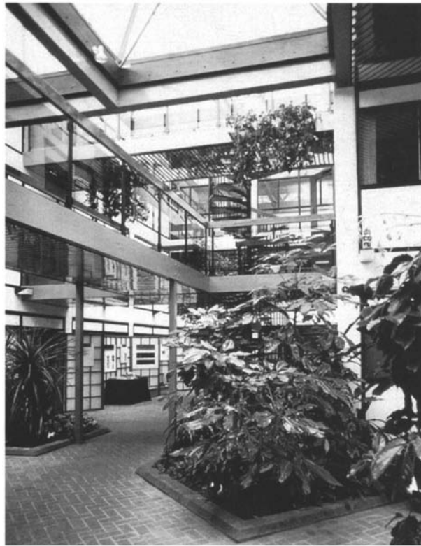
9.14 Unheated atrium at Cambridge Consultants Ltd maintains a minimum temperature sufficient for the tender but not tropical plants.
